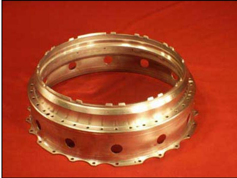
However, the following is the diffuser case design for the 757 jet engines and it is quite different from that shown at the Pentagon. That is due to the difference between "dual-chamber turbojet" versus the newer "high bypass jet fan" designs found on the 757 and 767 jet airplanes.
